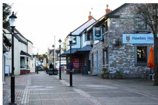
Historic buildings dating from the 19th Century and before are generally constructed from local stone or are rendered and painted white or pastel shades. Façades are characterised by sash windows, often painted white or a contrasting colour.
