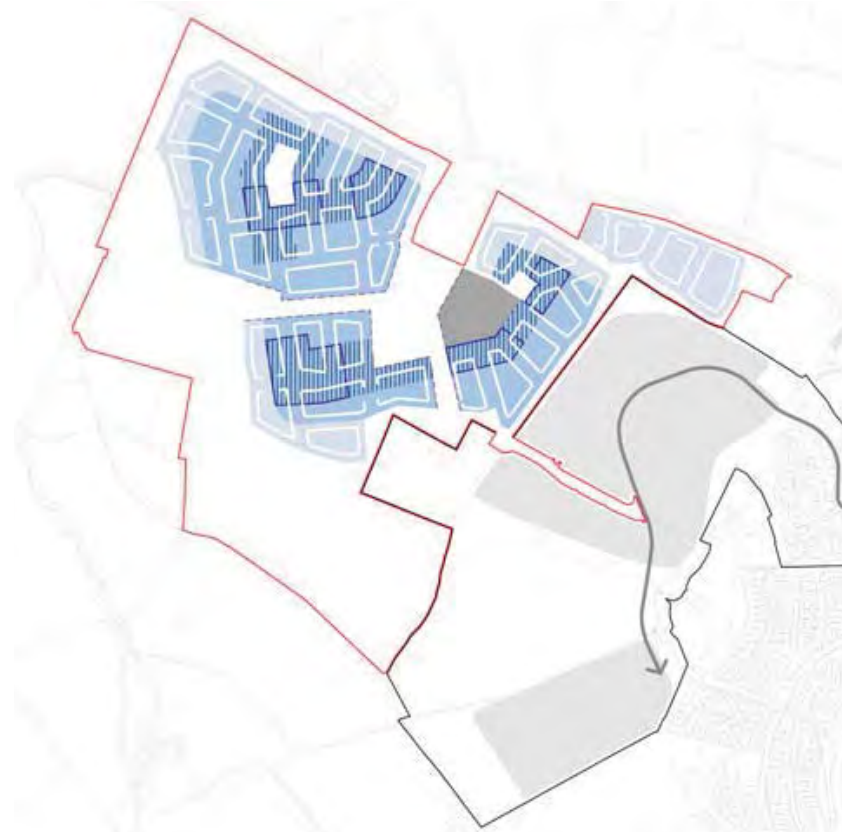
Above: Building height parameter plan with indicative development perimeter blocks overlaid to show how the maximum building heights relate to the envisaged masterplan structure.
