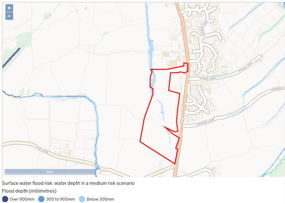
Figure 8: Medium Surface Water Flood Risk (Depth)
