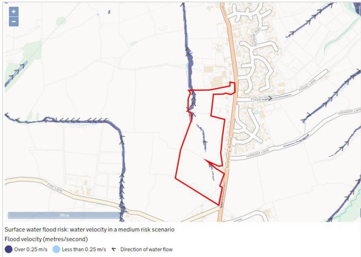
Figure 9: Medium Surface Water Flood Risk (Velocity)
