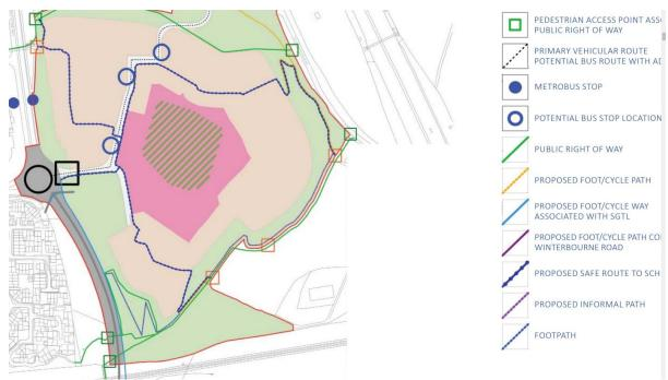
P21/06474/RVC allowed for the embankment to be redesigned here and the PROW moved to remove a retaining wall in this area but still provided a pedestrian link to the play area. The end of the roadway was shown as 62m AOD falling to 61m at the realigned PROW. An extract from the revised approved scheme 2331/hyb/017 rev M is shown below.
