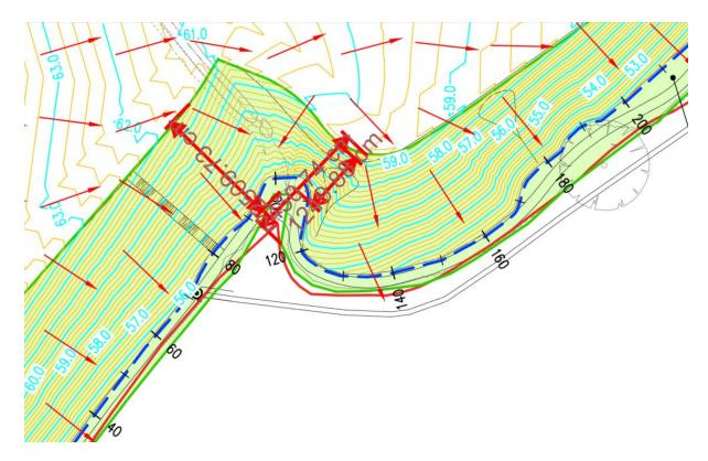
Proposed scheme tightens up the slope on this corner by moving the road by up to 4m, increasing the slope from 1:3 to 1:2.
