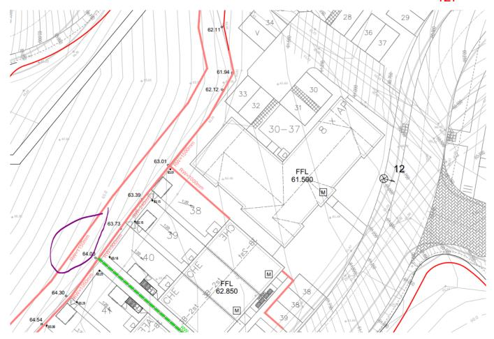
A foul pumping station is now proposed on approved POS, on a steep slope. It is proposed to be contained behind the 2.1m retaining wall. An approved POS path and planting would be obliterated by this proposal. Further details required.
