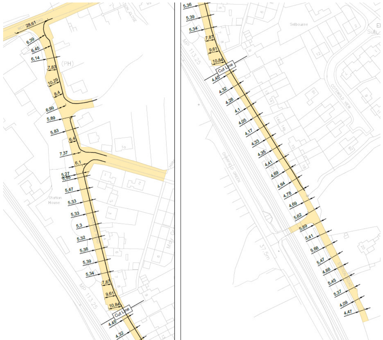
Figure 2: Station Road carriageway widths (not to scale) (Source: 2019 Ordnance Survey data)
